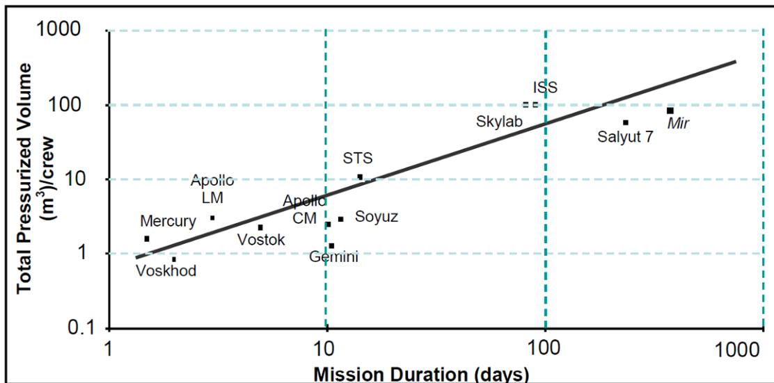
Figure 0.5: Spacecraft pressurized volume (NASA, 2010b p. 562, Figure 8.2-2)
