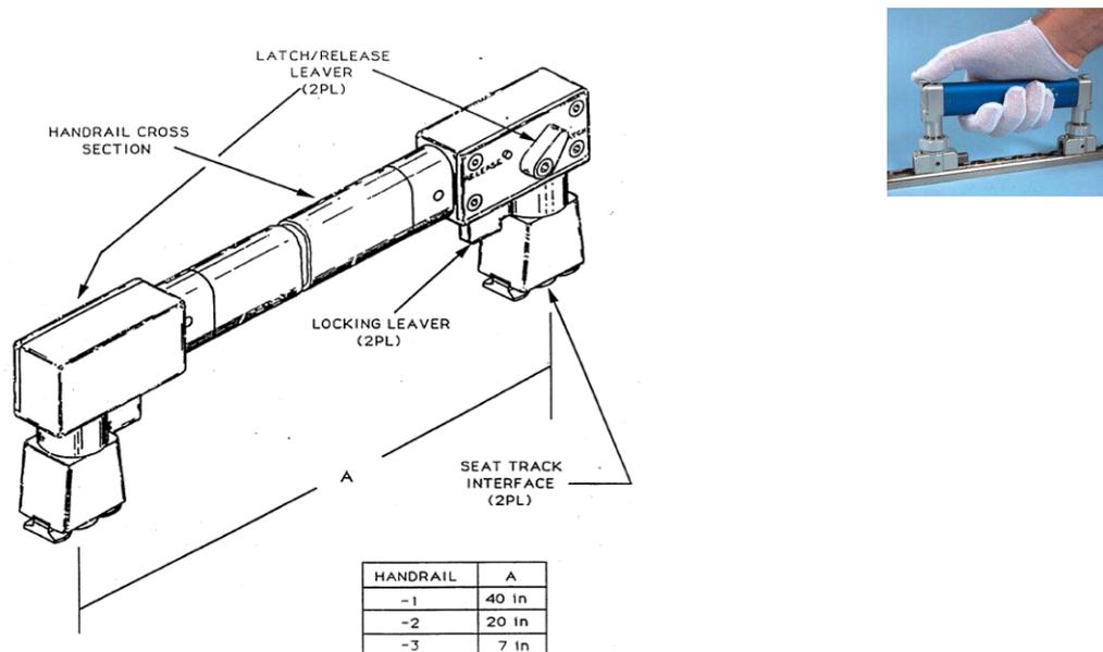
Figure 0.1: Removable ISS handrail (NASA, 2010b, Figure 9.7-1 p. 680; NASA, 1999 pp. 5-27)
