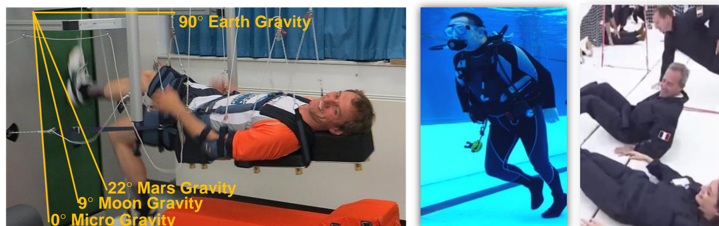
Fig. 3. Inclined Treadmill, Moon Buoyancy and Moon Parabolic Flight © DLR, NASA, ESA (Image elaboration Schlacht)
