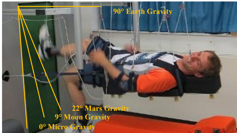
Fig. 6 Vertical Treadmill of DLR © DLR edited by Schlacht & Rittweger [11]
