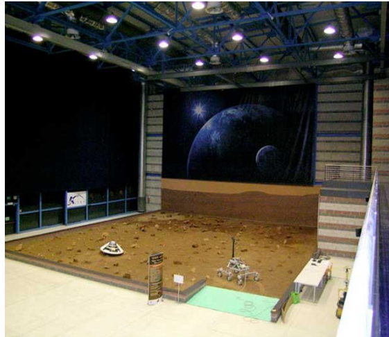
Fig. 7 ALTEC Moon-Mars Terrain for IVA test© LUNA consortium, visualization: Space Applications Services, 2015 [13]
