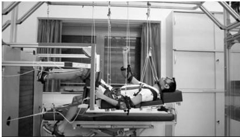
Figure 4: Mukadam self-experimenting Vertical Treadmill, © Mukadam 2017
