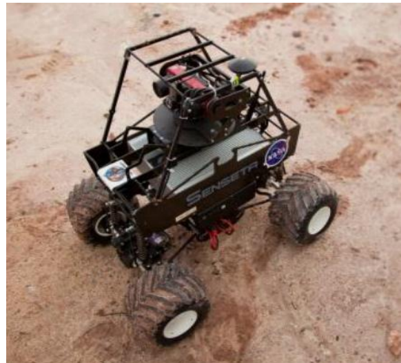
Fig. 1: Rover Senseta with dimension (cm) 46 x 38 x 42.
