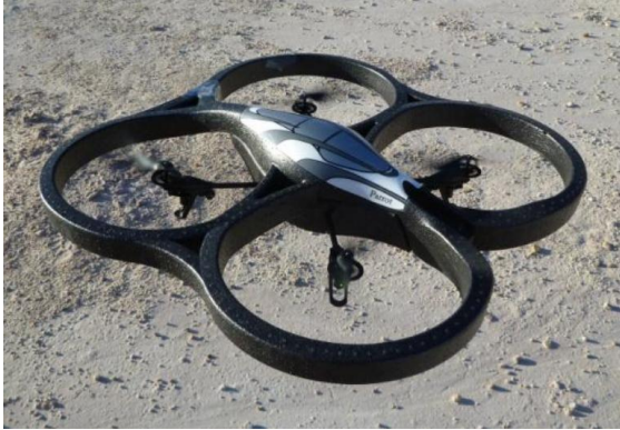
Fig. 5: UAV Parrot used during MDRS experiment to spot hazardous areas for the Senseta rover.
