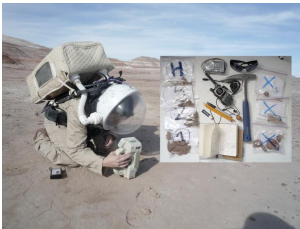
Fig.6: Problems with geological instrument interaction at MDRS, 2010: The instrument monitor is not visible because of solar light and helmet; the interface is not usable with EVA gloves; the instrument's design should be dedicated to the particular human-machine-environment interaction of space. It is not convenient to adapt earth instruments for use in space exploration.
